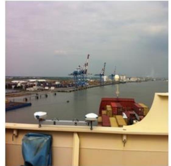
PPU installed on a ship bridge: courtesy of [Prácticos de Puerto](#)
