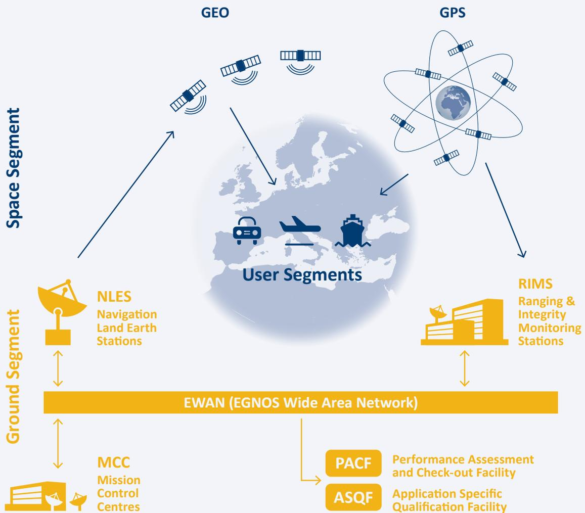
In order to provide its services to users equipped with appropriate receivers, the EGNOS system comprises two main segments: the Space Segment, and the Ground Segment.
