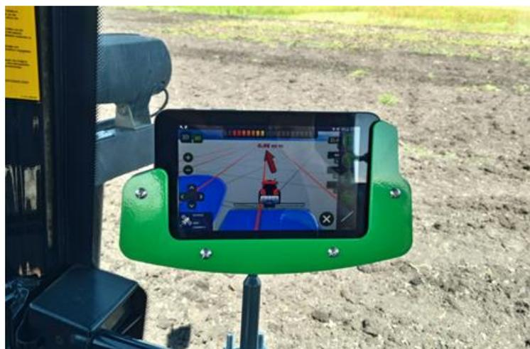
*Steering system installed on a tractor*
