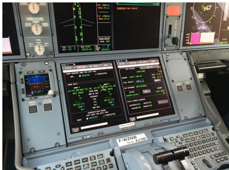
*Airbus350 flying a RNAV GNSS (LPV-200 based) approach*
