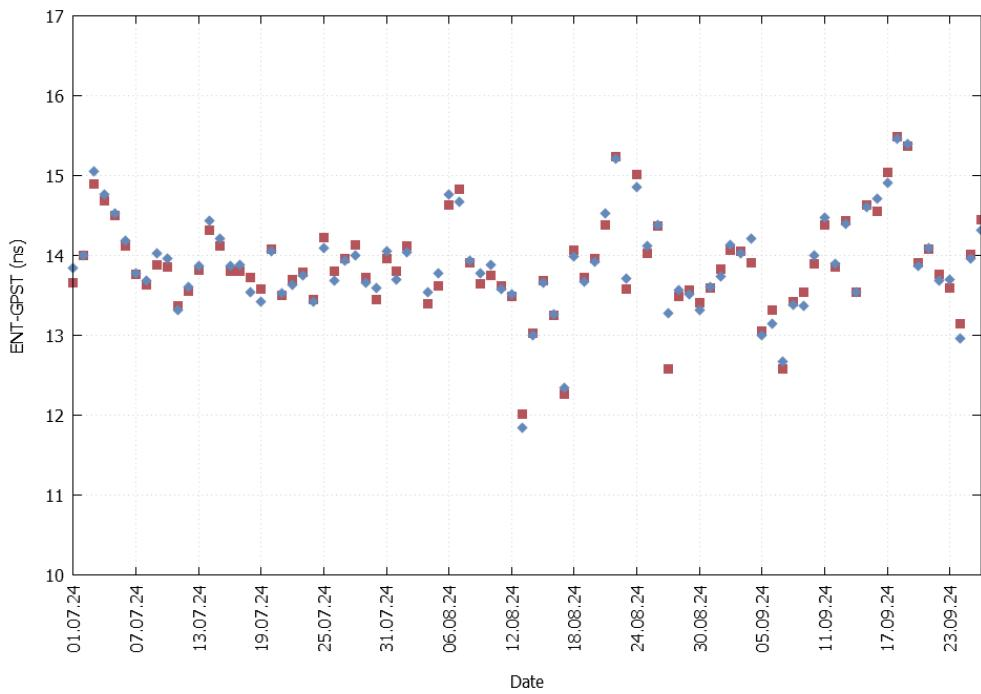
Figure 29 – ENT-GPS offset evolution from July 2024 to September 2024 (red PRN 123; blue PRN 136)
