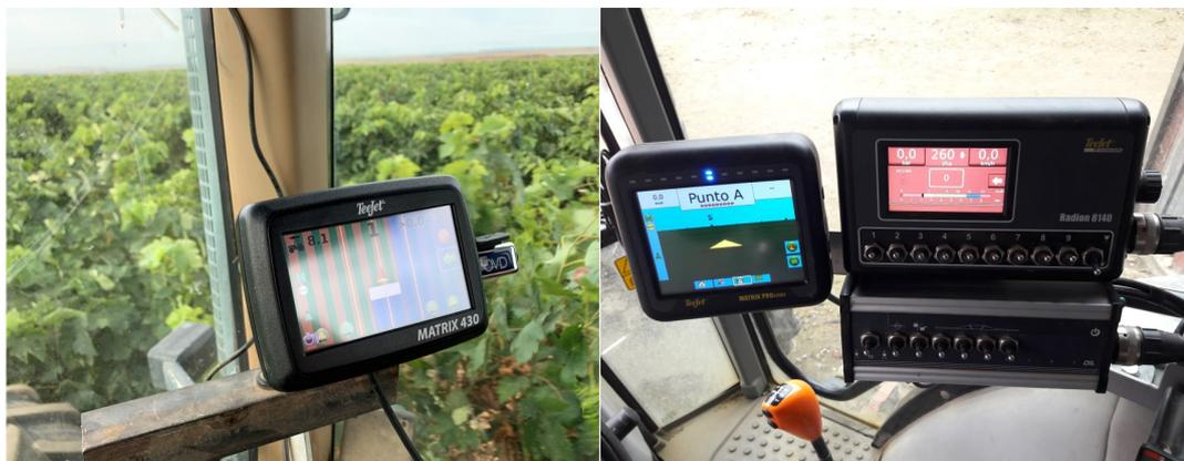
*Left: Tractor with an EGNOS-enabled guidance system from Teejet Technologies in action.*
