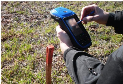
*Tracking control points in the field for soil mapping. CONAPA Courtesy*
